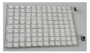
The LED System uses a Singular 4-SMD LED 24 Volt DC Modules attached together forming one light assembly.
