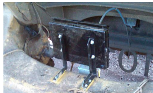
Rear Air Scoop uses Radiator Fan Air to keep Rear Screen Clean. c/w all Mounting hardware and LUNDKC Connecting Kit.
