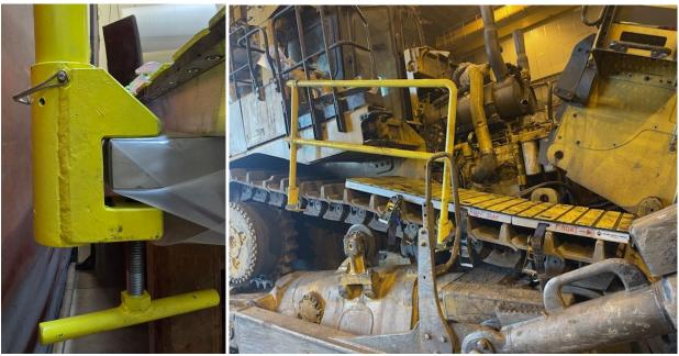
The DZMT HR was designed to provide a working platform with 42 inch hand rial for the safety or workers on large dozers. The extreme service hand rail clamp attaches securely to the track pad with an adjustable stanchion and hand rail to fit on any track pad. Each mat hand rail system can be converted easily to be used on left or right track.
